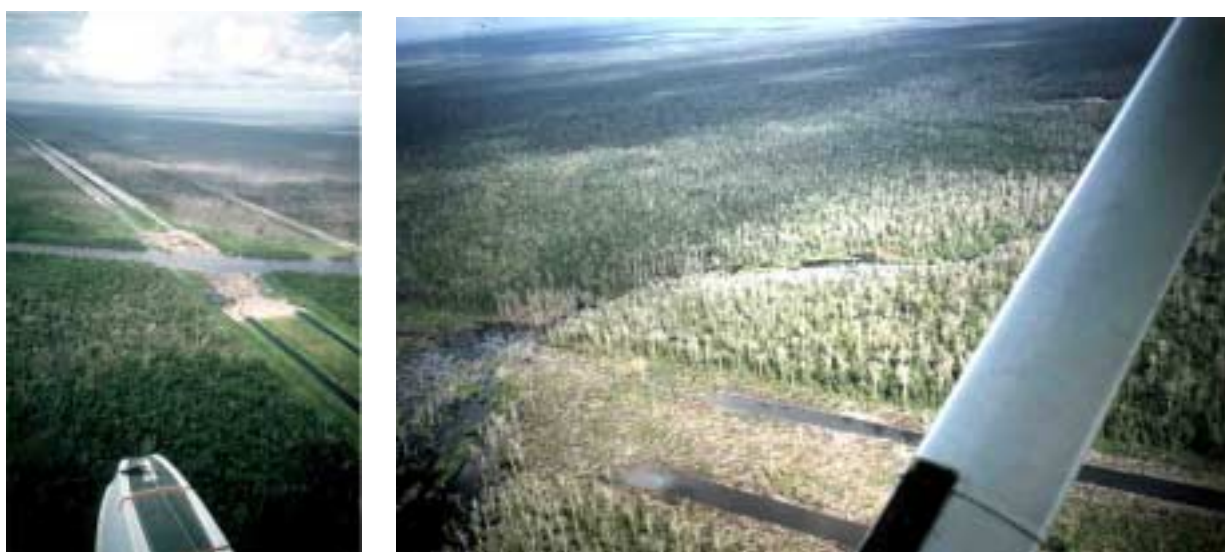
Fig. 10: Aerial photos acquired during a flight on 13 June 1998. A: PPC and burnt scars at Kapuas river with sluices, B: PPC interrupted by black water river Mentangai crossing the channels.
